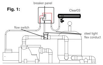
The ClearO3 unit is factory set to 240VAC. The ClearO3 should be wired to run with the filter pump which creates the air draw through the unit needed to create ozone. Do not set the ClearO3 to run when the filter pump is off.
