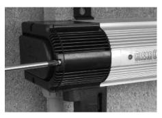
Turn the power off to filtration system pump at circuit breaker. Remove three screws in left end side cap labeled "electrical connections".
