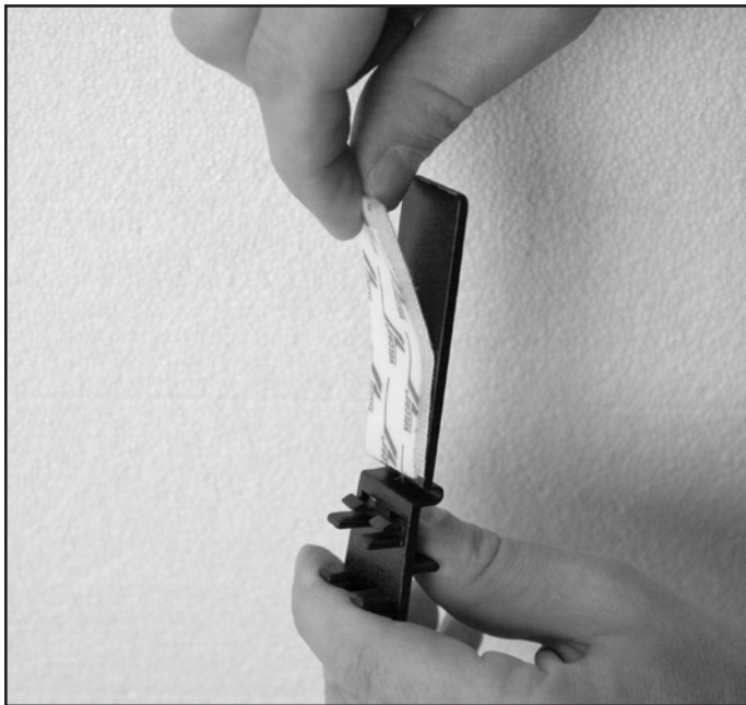
Diagram 20 - Velcro tape on Upper Tabs
