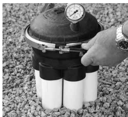
8. While tightening band clamp, lightly tap clamp with a screwdriver or wrench
