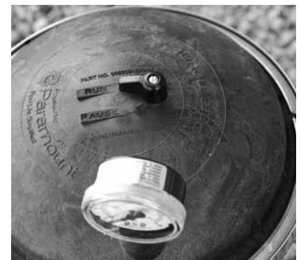
7. Turn water valve to "RUN" position
