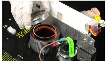
7. Grip quartz tube with both thumbs inside and pull up. Once the O-ring breaks free, the quartz tube should lift out easily. Fig. 13
