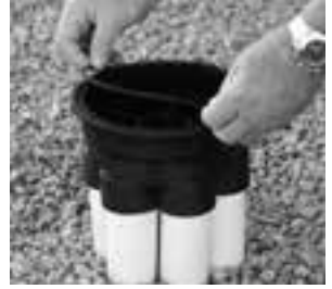
3. Clean and install base o-ring
