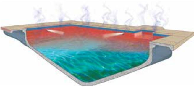
Ordinary pools circulate water near the surface where chemicals and heat are quickly lost into the atmosphere. This wastes chemicals, heat energy, and can create algae-prone areas due to poor circulation.
