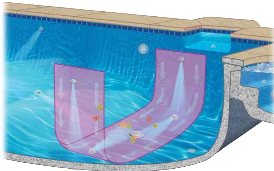
Strategically placed fixed nozzles and downjets direct debris into the MDX-R3 main drain
