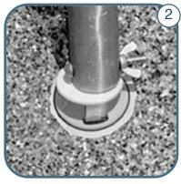
Use removal tool made for existing nozzle to remove one nozzle at a time by rotation 1/4 turn counter clockwise to unlock. The system is hydraulically balanced, so the same size nozzle needs to go back into the appropriate hole.
