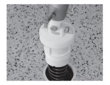
4. Press the top of the complete RetroJet nozzle onto the three prongs of the RetroJet installation tool\*. Guide the nozzle into the hole in the pool floor and then rotate clockwise 1/4 turn to lock in place. Allow the nozzle to cycle through the cleaning process to ensure that it was installed properly.
