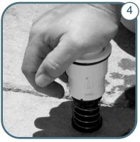
Place the selected cap over the the top of the RetroJet nozzle and press firmly against a hard surface. You will hear a snap when the pieces have properly locked together.
