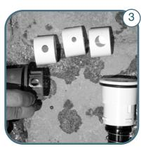
Check the size of the opening on the existing nozzle and then select the closest RetroJet cap from the pack of three provided in the replacement kit.
