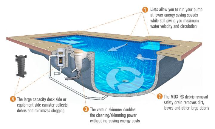
Four exceptional products work together to create the most effective and efficient circulation in pools with multi-speed and variable speed pumps
