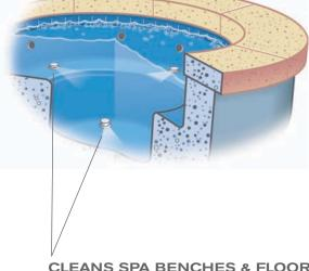
POP-UP CLEANING JETS MOVE DEBRIS OFF THE BENCH TO THE POOL FLOOR WHERE THE ROBOTIC CLEANER CAN REMOVE IT.
