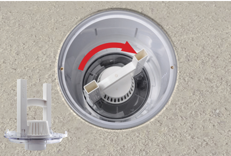
3. Insert MVFUSE lid assemble into canister. Turn lid assembly clockwise until it clicks into place on the retention stops.
