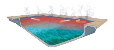
Pool without Cyclean in-floor system is poorly circulated, resulting in chemical and heat energy loss, as well as algae-prone areas
