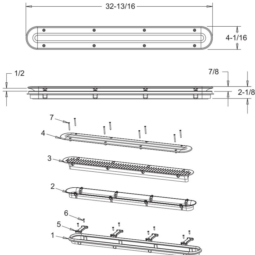
1. 32" channel drain, no sump, frame
