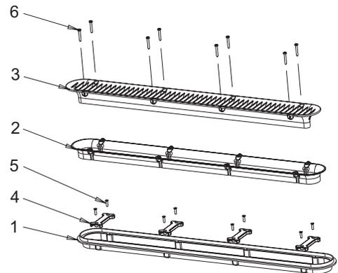
1. 32" channel drain, no sump, frame
