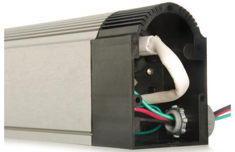
Press plug onto light bulb. Replace side cap and three screws. Turn on power to filtration system pump.
