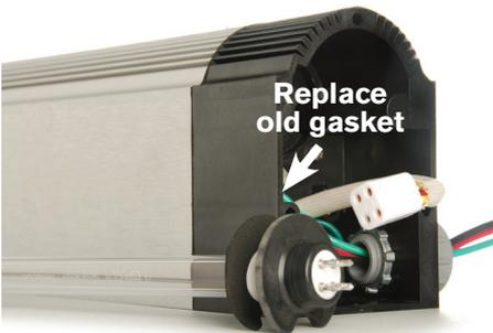
Remove and throw away the old gasket. Make sure new gasket is in place on replacement bulb. Align with key and slide into hole until bulb is completely into unit.
