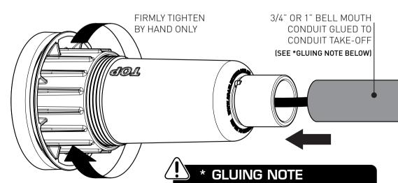
ENSURE P.V.C. SOLVENT CEMENT IS SUITABLE FOR NON-PRESSURE APPLICATIONS AND USE WITH A.B.S. PLASTIC
