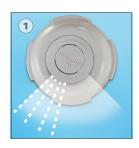
The nozzles are installed as wall returns and are hydraulically activated to pop out and deliver a high-pressure stream of water.
