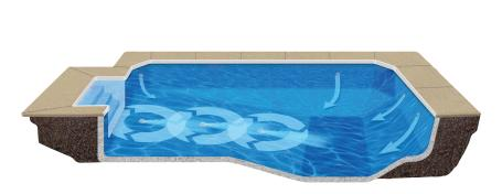
Pool without Vanish in-floor system is poorly circulated, resulting in chemical and heat energy loss, as well as algae-prone areas
