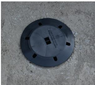
**1.** Before pouring concrete around the Vanish™ body be sure the cap is on the body. Pour concrete in a 12"x12"x6" deep area and trowel smooth with the flange on the body and the finish level of the vermiculite. Be careful not to get concrete in the screw holes.
