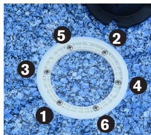
**6.** Rotate the installation tool, press down again and install remaining screws in the order shown above.
