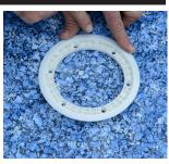
3. Align the clamp ring over the body. There are 3 bumps on the body that corresponds with notches in the clamp ring (see step 2).
