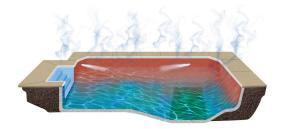
Pool without Vanquish in-floor system is poorly circulated, resulting in chemical and heat energy loss, as well as algae-prone areas
